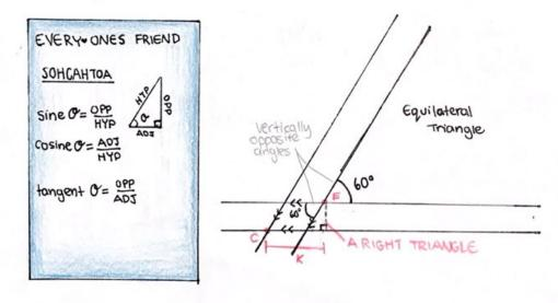
To solve for length k, I would need to find the lengths a and b by trigonometry. Using cosine, length a can be solved as the adjacent side of the triangle from the 30° angle is 1 ft and the hypotenuse (x) needs to be found. This gives the equation  $\cos 30 = \frac{1}{x}$  so  $x = \frac{1}{\cos 30}$ . Solving for length b, simply uses Pythagoras. We know the hypotenuse and one side length—thus side length b would equal
